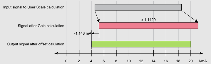
Fig. 6: Value range offset from the range 4.5 mA to 18.5 mA to the range 4 mA to 20 mA
